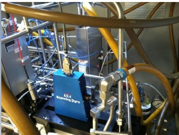
power connection. Attached to the optical head and supported by the mounting hardware, the motor controls the scanning of the optical head across the slit. The optical head has one connection to the control computer.
