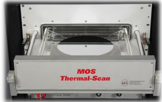
Vacuum heating chamber for up to 200mm diameter wafers.
