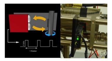
properly tracked and utilized within any kSA product to define measurement positions. Custom mounting brackets are typically required for individual needs and can be manufactured at additional cost.
