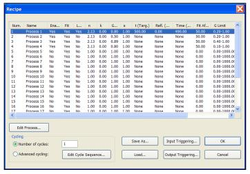
Recipe Table: The recipe table allows the user to see all the processes that have been programmed. Each process can be programmed to look for a target thickness, reflectivity, and a time limit. The system will output a TTL level signal to indicate that a process has been completed.
