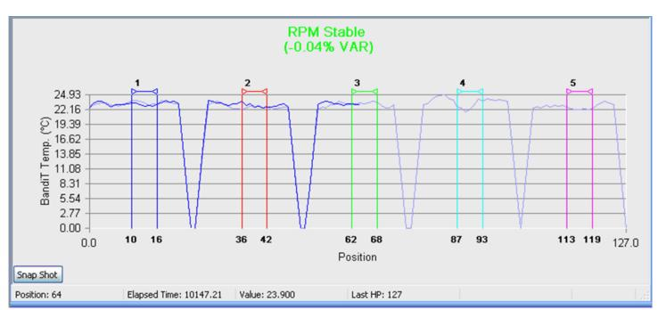
kSA RateRat uses signal intensity changes in the wafer and carrier to visually trace and define wafer positions during rotation. The user is then able to accurately place measurement "markers" at any position to enable real-time monitoring that location. Wide markers are available when averaging over a particular wafer or carrier area is desirable for process control. Up to 180 markers may be placed within or across multiple wafers.
