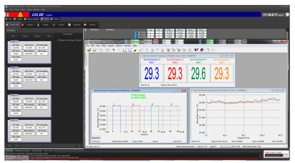
This kSA BandiT screenshot shows the real-time temperatures for the four selected markers, the band edge temperatures of the markers over a full rotation, and the band edge temperatures over time. It overlays Crystal XE's System View, which displays the kSA BandiT data in real-time. It can be customized to display other real-time data as well. The start, stop, pause, and resume buttons allow for easy control of kSA BandiT data acquisition from Crystal XE.
