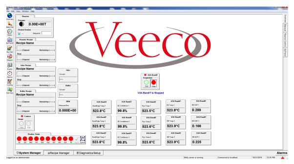
This Molly screenshot illustrates the integration of kSA BandiT. It shows band edge temperature, band edge fit confidence, pyrometer temperature, blackbody temperature, and blackbody goodness of fit for three selected markers. It can support up to 20 markers. The start and stop buttons allow for easy control of kSA BandiT data acquisition from Molly.
