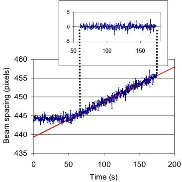
Figure 4. Beam spacing during epitaxial growth of  $In_xGa_{1-x}As$  on GaAs(100). Growth is initiated at t=50 s at a rate of 0.23 nm/s. The red line corresponds to the best fit for growth of a film with constant stress. The difference between the measurement and the fit is shown in the inset.
