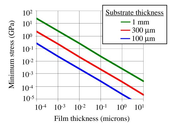
Figure 7. Sensitivity of MOS system for different film and substrate thicknesses. The modulus used for these calculations is 100 GPa and the minimum resolvable value for  $\delta d/d_0$  was taken as 0.05%.
