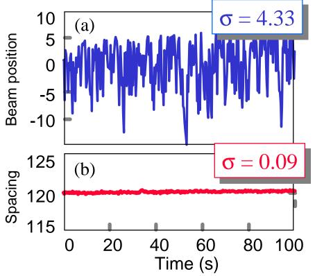
Figure 6. Reduction of noise during *in situ* curvature measurements by using multiple beams. a) Relative position of one of the MOS beams in units of pixels. The RMS deviation of 4.33 pixels is caused by sample vibration. b) Measurement of the spacing between adjacent MOS beams taken at same time as data in (a). The RMS deviation is 0.09, much lower than the single beam measurement.
