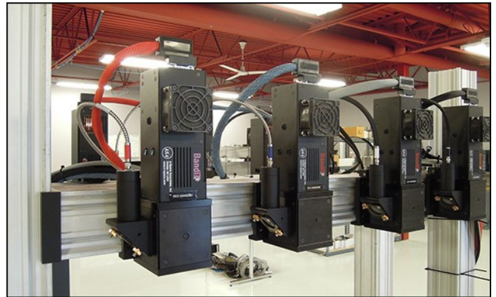
Figure 11: Yes. kSA BandiT PV Thin Film Process monitor with 4 heads.
