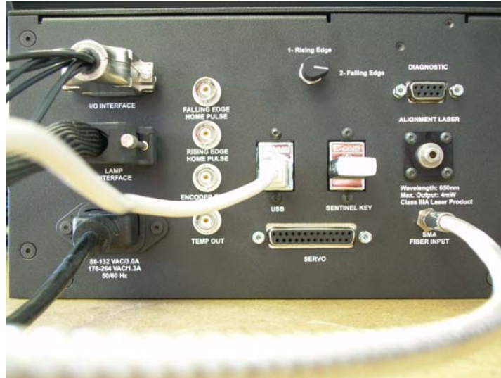
Figure 10: Rear Panel Cables Connected
