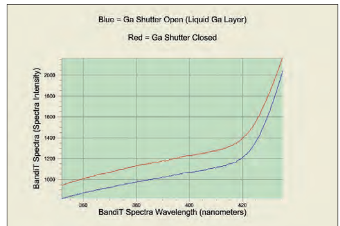
Diffuse scatter signal decreases with Ga liquid layer formation during MBE GaN growth
